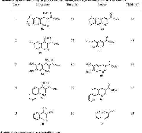
TABLE 2. Quinolines Synthesized by [Cp\*Fe(CO)<sub>2</sub>]<sub>2</sub>-Catalyzed Cyclization of BH Acetates
